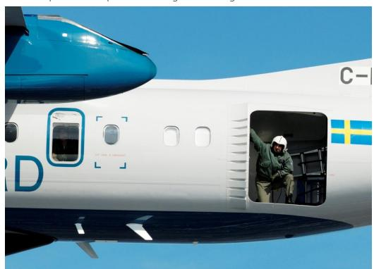
The AOD utilizes the existing inward-opening, plug-type OEM cargo door, which is modified to add an internal handle for opening and closing the door. Other modifications include an attachment point for two crew members, non-slip flooring and a fuselage mounted air deflector.
